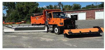
Courtesy of the Vermont Agency of Transportation The new Magna "Wing" truck with a 21-foot wing for plowing Vermont's busy Interstate 89
